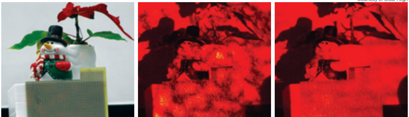
The scene (left) is illuminated with a helium-neon (HeNe) laser with no speckle reduction (center) and with a HeNe laser with speckle reduction (right).
